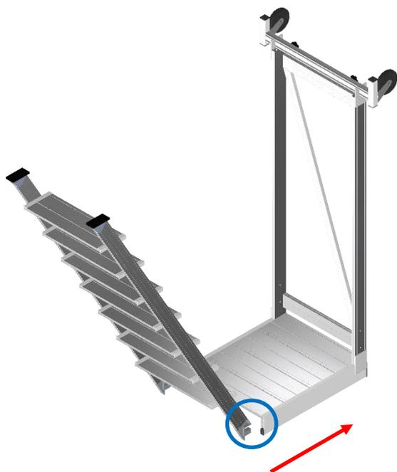
4. MONTARE I DUE SOSTEGNI DEL DISPOSITIVO ALZA SCALA, SULL'ALZA-SCALA. SUCCESSIVAMENTE MONTARE IL DISPOSITIVO ALZA-SCALA SOTTO LA SCALA DI SALITA, SVVITANDOLO AI FORI POSTI APPPOSITAMENTE SUI MONTANTI.
